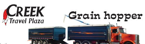
A grain hopper is a trailer pulled by a semi-tractor and used to haul bulk commodity products. Theses trucks are used extensively throughout the U.S. to transport agricultural products as well as any other commodity that can be hauled in bulk and loaded and unloaded through the trailer.
