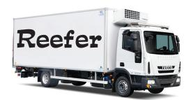
Reefers are those that have a refrigerated unit built directly on the truck frame or is transported by a trailer. These trucks deliver a vast assortment of things that need refrigerating. The most common item seen in reefer trucks is ice cream, but reefers also transport human organs for transplants, blood and plasma, flowers and much more.
